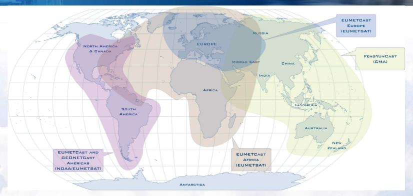
Multi-service dissemination system based on standard Digital Video Broadcast (DVB) technology. It uses commercial telecommunication geostationary satellites to multicast files (data and products) to a wide user community.
